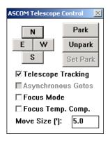
The "Telescope Tracking" check box allows the tracking to be turned off or on. The "Asynchronous Gotos" check box determines how telescope "goto" commands work. If checked, when "goto" commands are given, the telescope will start to move and control is returned to **ECU** almost immediately. If not-checked, then when "goto" commands are given, **ECU** waits (with an hour-glass style mouse cursor) until the "goto" operation is complete before regaining control.
